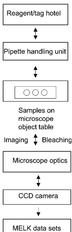
FIG. 1. Schematic illustration of the imaging cyclus set up running MELK procedures.
